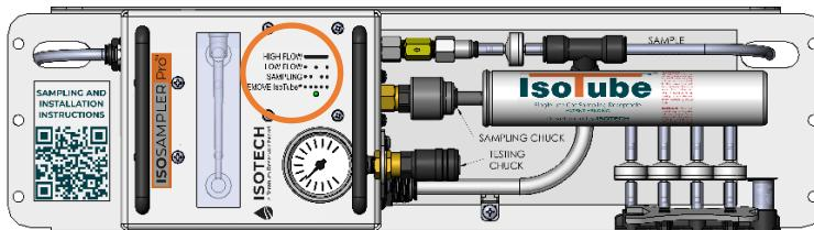
When the pump stops running and the LED starts to fast flash remove the IsoTube from chuck.
